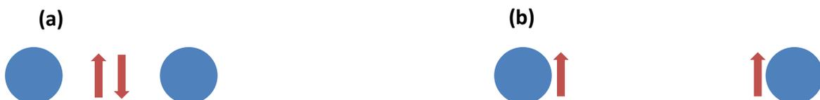
Figure 2.3: (a) Antiparallel alignment for small interatomic distances, (b) Parallel alignment for large interatomic distances.
