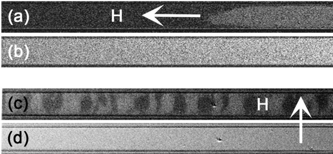
Figure 4.14: Evolution of magnetic domains for different field orientations.  $\phi_H = 0$ , a) appearance of large single domain, b) fully saturated wire.  $\phi_H = 90^\circ$ , c) appearance of multi-domain, d) fully saturated wire. The arrows show the direction of applied magnetic field.
