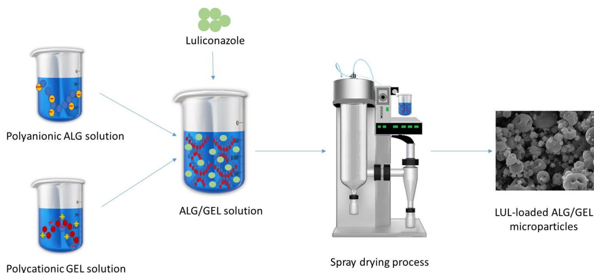
Figure 1. Scheme for LUL-loaded ALG/GEL microparticles preparation.
