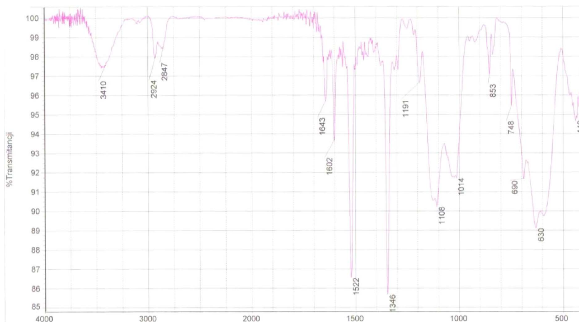
Fig. 6. ATR FT-IR spectra of MNPs@N = CHC 6 H 4 NO 2 nanoparticles.
